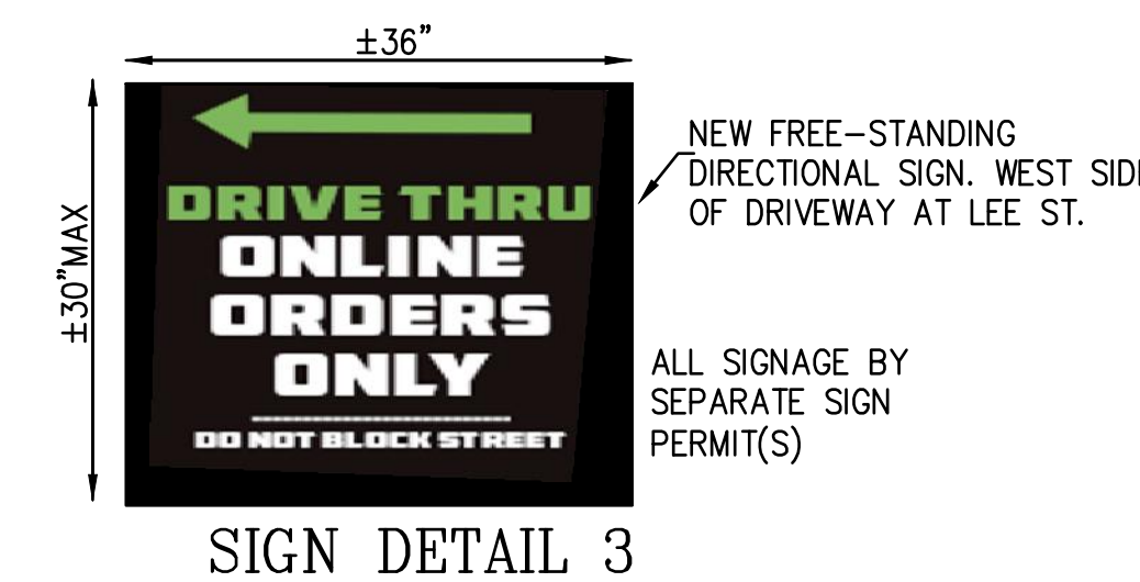
NEW FREE-STANDING DIRECTIONAL SIGN, WEST SIDE OF DRIVEWAY AT LEE ST. ALL SIGNAGE BY SEPARATE SIGN PERMIT(S) SIGN DETAIL 3
